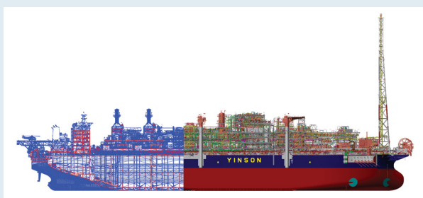
Concept illustration of an FPSO digital twin
